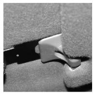
Loosen (or remove if necessary) both visor clips for the 274-ULB21-U1 or the passenger side visor clip for the 274-ULB10-U1. They should be loose enough that one of the forked brackets can easily slide under each clip, then tighten the clip such that it securely holds each bracket in place.
